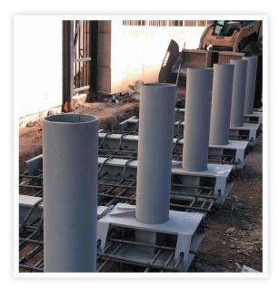
**Bollard Design and Manufacturing** - The Bollard design required numerous individually fabricated pieces to fine-tune the aesthetics and lighting implementation prior to production.
